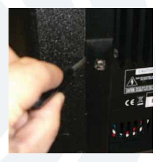
The covers may be worked loose by wedging a flat head screwdriver in between the cabinet and the cover, as well as the amplifier assembly and cover. Make sure to get around the entire cover plate in order to be able to remove them.
